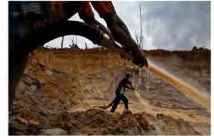
Hydraulic mining known as 'chupadeira system' a form of mining that uses high-pressure jets of water to dislodge rock material or move sediment is being used in an Agua Branca gold mining village, Para State, Brazil.
